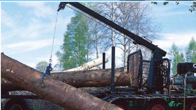
The log loading is easily done with the heavy duty loader crane and power winch. Lifting capacity is 300 kg.
